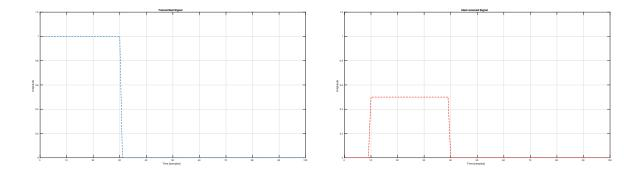
We plot both the ideal TX and RX signals in order to evaluate easily what are the shape modifications due to noise in the second part of this exercise. For the ideal RX signal we have just applied an attenuation of amplitude that could be modelled as a typical free space loss.
